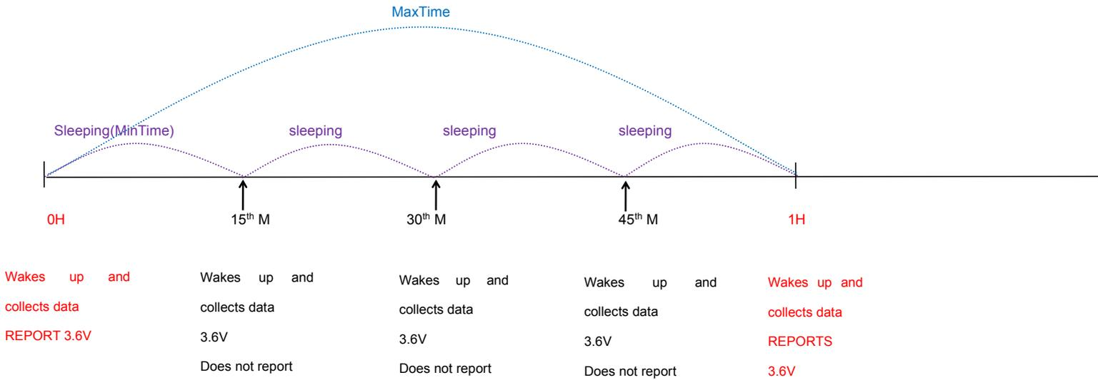
**Example#3** based on MinTime = 15 Minutes, MaxTime= 1 Hour, Reportable Change i.e. BatteryVoltageChange= 0.1V.
